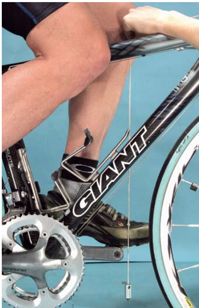
The saddle here is either too low or too far forward, placing the knee in front of the pedal spindle, hence increasing flexion and loading the PFJ.
